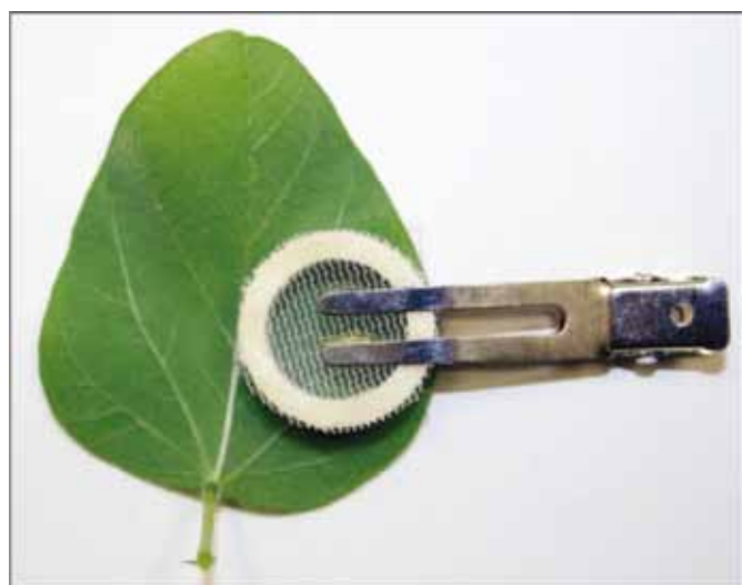
A clip cage to measure growth and development of single aphids.
